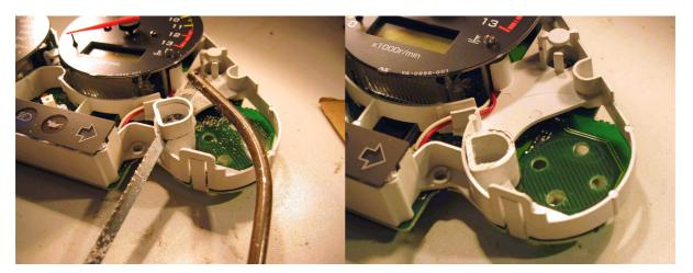
9.) Pull all the cables from the gear indicator through the resulting hole 10.) Tighten the screws (supplied in little plastic bag) to secure the unit
