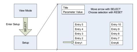
To move the cursor press and hold the SELECT button until the arrow cursor moves to the desired position. To then select a menu item press the RESET button.
