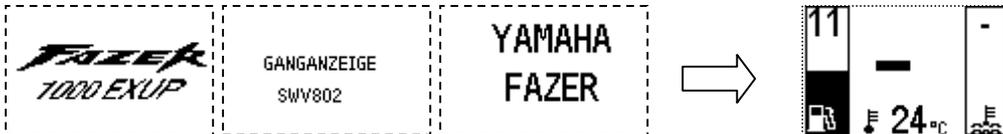
At standstill the electronics is not able to determine the engaged gear as no speedo signal is available. This state is indicated by a horizontal bar.
