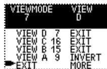
The small indicator arrow can be moved by pressing **S**. The headline displays the last active state before entering the menu (example: favorite D assigned to viewmode 7). The next example moves the indicator to VIEW C and alters the value from 16 to 1 by pressing **R**:
