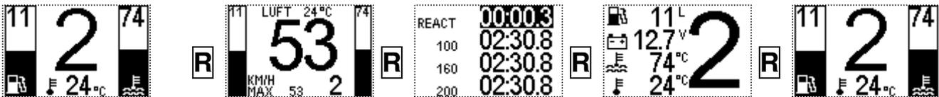
At power-up the display is always set to the first favorite (VIEW A). The mapping of viewmodes to favorites is not restricted, also multiple usage is possible. A very easy and comfortable way for switching is the installation of a „third button“ (**3**), e.g. by converting the flash light button.
