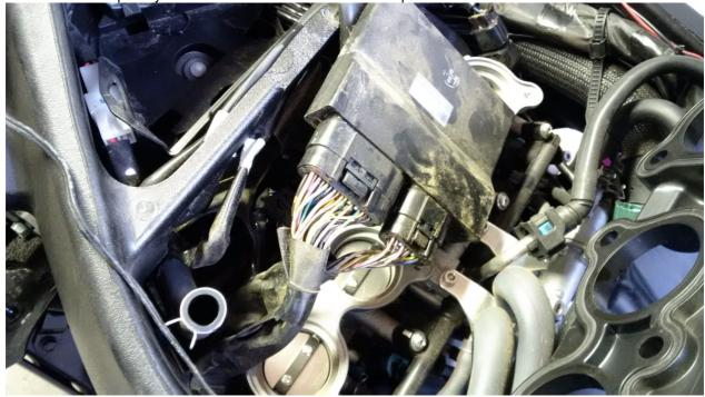
Open the isolation tape to get better access to the wires.
