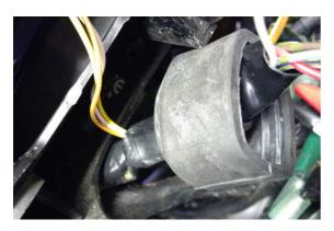
Remove the backside of the dashboard compartment. Solder the wires to the designated spots on the main board. Don't forget to route the wires through the opening in the backhousing before! "Button" is connected to RESET.
