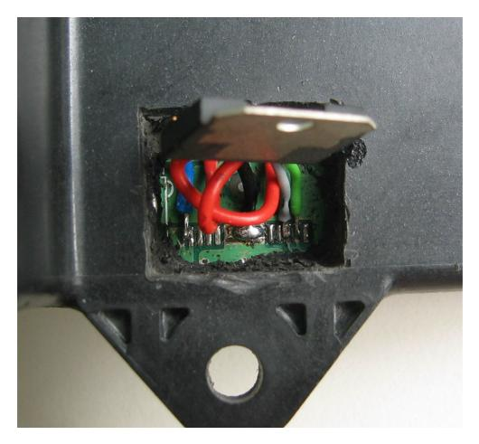
Push the new IC into the cavity and seal it with some epoxy glue. Try to restore the original surface height (or lower) as the ECU rests on the lower side.
