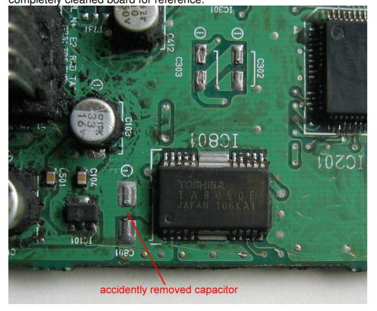
Replace IC801 with a new TA8050F. The ground flaps might be hard to solder.
