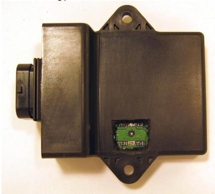
IC801 is the servo controller. Be careful to not damage any nearby parts. See this completely cleaned board for reference.
