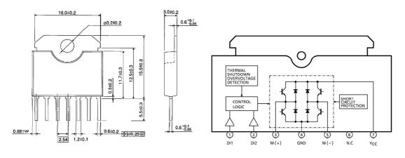
Caution: Swap M(+) and M(-) when replacing the TA8050F with TA8050P! Same naming but reversed logic.
