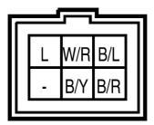
B/Y, B/R: Motor connect 12V and ground for testing
